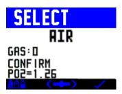
Selecting the tick returns you to the Home screen if on the surface or the dive screen if underwater and you gas selections are all saved. Selecting allows you to go back through the adjusting sequence again or selecting allows you to switch to closed circuit mode (if you have the PIN installed).
