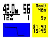
If XDec is set to YYY and XFunc is set to 3xO2 then all three sensors and the average PO2 (x1.15) will be displayed. An x (x1.15) denotes that the external cell reading is being used.
