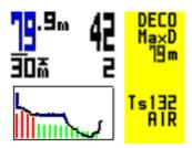
and can be used to display the dive graph, or the Total Time to Surface (TTS), or external PPO2 (if the external triple or single cell option is enabled) or a combination of the above. To make your choice, go to the Gmode option in the Display Options. The modes are:
