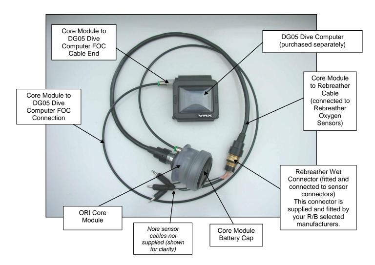
**NOTE:** Hollis Gear can supply the rebreather wet connector to rebreather manufacturers and approved service centres ONLY. They will fit and test the connector and ensure the correct interfacing to the rebreather's existing control system. The core module to rebreather cable then simply plugs into the fitted wet connector.
