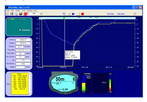
The decompression information is shown in the bottom left corner of the dive display window. When there are stops, the window background is set to yellow.
