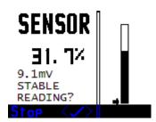
With a short push of both buttons you will be prompted to **Flush** the cell with the cal gas, then **Equalise** the pressure (ensure no excessive flow or a closed mouthpiece in the case of a rebreather sensor calibration can put extra pressure on the oxygen sensor). Then you will be asked to confirm that the reading is **Stable**.
