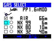
Now a short push of both button moves along the gas row and allows you to change a function/% by using the - and + buttons. If you change the MOD the PO2 of the selected dive gas will also change.
