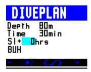
Once you have set your planned dive gases in the DG05. Diveplan allows you to enter depth, time and surface interval and calculate a set of backup tables. The current decompression used for planning is shown.
