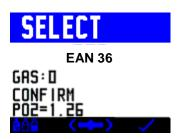
This will take you into a screen where you will see the new gas you wish to switch to based on the MOD of that gas and the plan you entered. A short push on the right switch will then take you back into the dive screen where the new gas will be displayed and decompression will begin to be calculated based on this gas.
