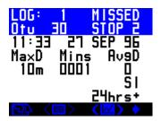
The logbook screen shows depth, time and surface interval information as well as accumulated OTUs (oxygen tolerance units). If a decompression stop is missed or violated during a dive, the MISSED STOPS warning is displayed in the top right corner of the screen. If multiple stops have been missed, the number of stops missed is shown immediately after the word STOPS.
