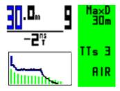
**AvgD** – The average depth feature when selected displays the current average depth based on the dive profile thus far. It is displayed in the right hand side of the dive screen. Some training agencies use the Average Depth decompression system, with dive tables to calculate decompression. The advantage of using it with a decompression computer is that you can cross check your calculated results and have a back up in the event of a tabular mistake.
