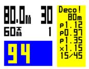
Note: if the partial pressure of oxygen in the diluent at the prevailing dive depth exceeds the DG05's internal set point, then the diluent PO2 will be displayed instead of the set-point.
