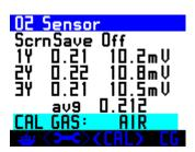
On this screen (and also from XDec in the Dvo screen, if XDec is set to YYY) you can disable <D> faulty oxygen sensors by pressing and then to move around the screen and then <D> to disable each sensor. This can be done while submerged (in Dvo) or at the surface (cell mini screen or Dvo). By doing this the average reading will be modified.
