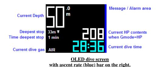
**Gmode** can be set to HP (if fitted), TTS or PO2. PO2 is only available if a DG05 rebreather interface (ORI) is fitted.
