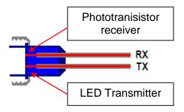
FOC is flexible and robust but it can break. However, small cracks will still allow data to pass through and water can even assist in transmission since it fills the cracks better than air, allowing light to pass. The supplied FOCs are extra-long to allow for trimming after accidental breakage. From a service perspective, replacement cables are relatively inexpensive, and can be sent easily by post or retained in a spare parts kit.
