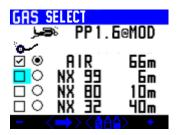
Now a short push of both button moves along the gas row and allows you to change a function/% by using the - and + buttons. If you change the MOD the PO2 of the selected dive gas will also change.
