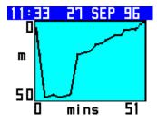
The DG05 has a second log screen, accessible by a long push of both switches, in which a graphic profile of the dive is shown. While in the graphic profile screen, a short push of both switches will bring up a screen showing a graph of ambient temperature throughout the dive.
