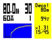
In closed circuit mode with an external cell connected and XO2 set and XDec ON the actual from the external cell PO2 is shown on the second line up.
