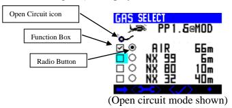
There is a square function box and a radio button. In G3 mode only 4 gases are displayed. In G10 mode by using the left button all 10 gases can be displayed on extra screen pages.
