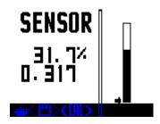
The PO2 bar graph has no digits but the bottom of the bar is zero and the top 2.0. The small arrow to the left of the bar represents the DG05's internal PO2 set point.
