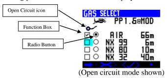
There is a square function box and a radio button. In G3 mode (see Setup screen) only 4 gases are displayed. In G10 mode by using the left button all 10 gases can be displayed on extra screen pages.
