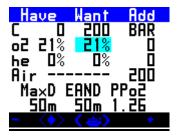
You have the option to purchase a PIN to activate this feature. When this mode is enabled, you can gain access from the Home Screen, (toggle through the miniscreens). Gas Calculator mode will allow you to work out partial pressure gas fills on your DG05.
