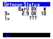
The Optocon connection system allows a range of sensors to be connected to the DG05. As this is an infra-red system there are no electrical connections as such hence there is nothing to become corroded as with conventional wet connectors. Having connected up the relevant interface the DG05 will automatically set the XFunc mode to suit the interface. If an oxygen sensor(s) is sensed XFunc will automatically select 3 sensor mode, you can then change this back to one sensor is required.
