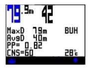
When exiting the dive plan (long hold both buttons from the dive screen), the equivalent gradient factor is displayed:
