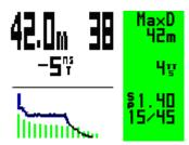
In closed circuit mode with the external sensor XO2 set and XDec OFF, the PO2 setpoint is displayed on the second line up in the right hand section of the screen.
