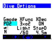
To allow calibration of the O2 cells, the O2 sensor screen below will be shown if XFunc is set to 3xO2. These screens are accessible from the main dry mini screen menu entitled 'O2 Sensor' and reached after a short push of both buttons (<GO>).
